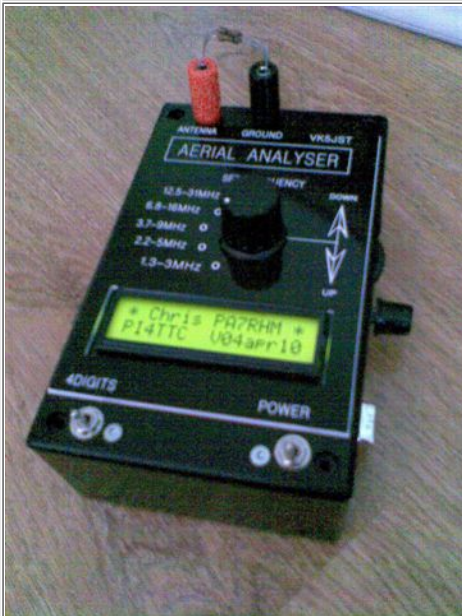
Chris's Analyser complete with additional comport on the right side of the box.
