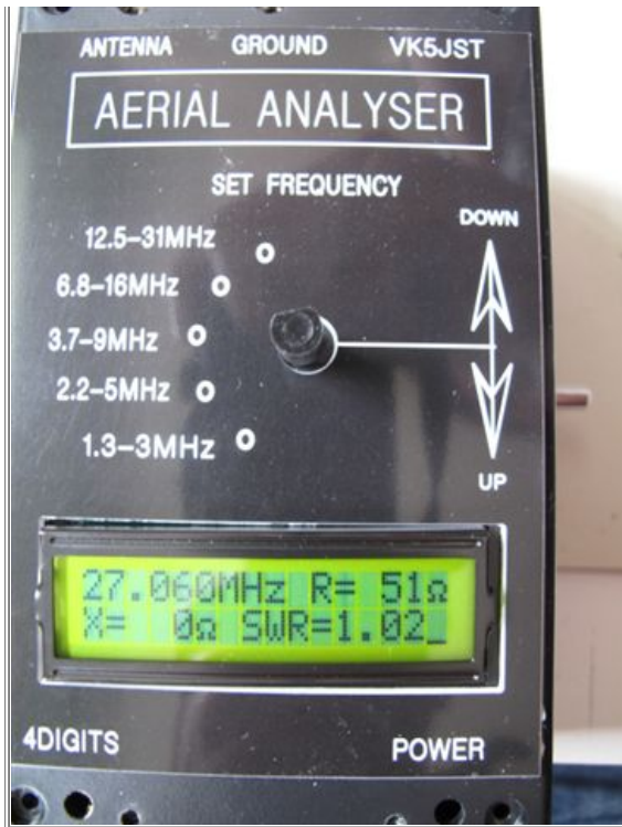
Chris's Analyser complete with additional comport on the right side of the box.
